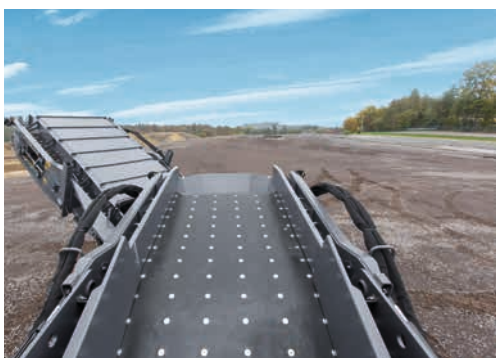
Flexible in use – the optionally available swivel belt with 6.5 m (OC 650) for BMF 2500 S.
