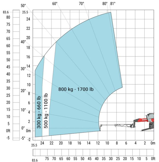
Machine on lowered stabilisers with hook 6000 kg (Metric)
