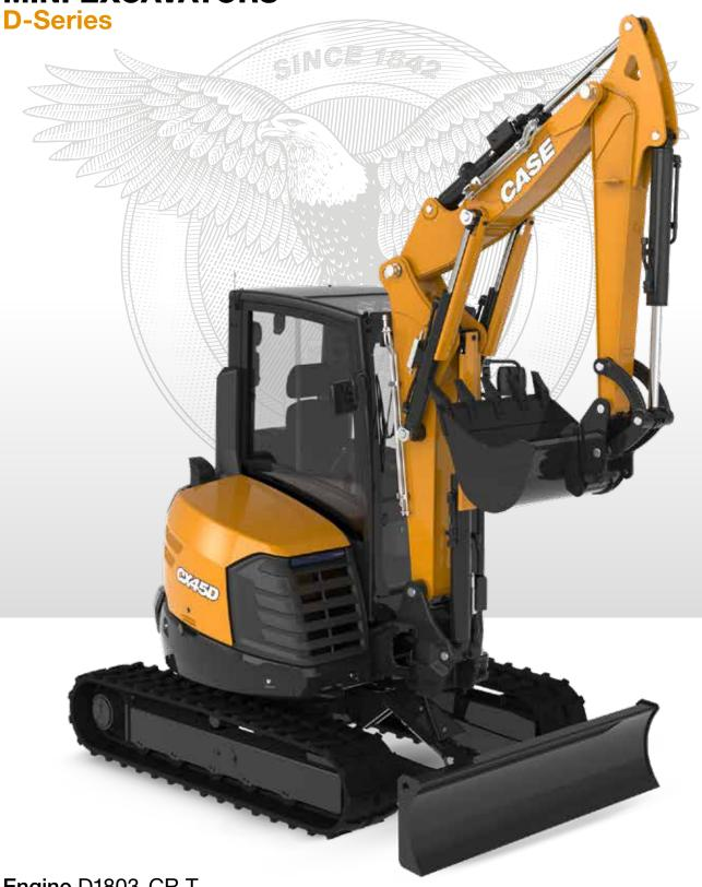
Engine D1803-CR-T Engine power 32.3 kW - 43.9 hp Operating weight 4750 kg
